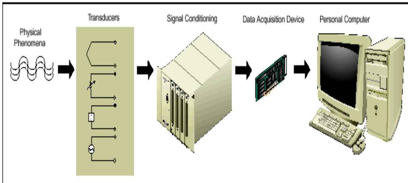
One of the most common signal conditioning functions is amplification. For maximum resolution the voltage range of the input signals should be approximately equal to the maximum input range of the A/D converter.
