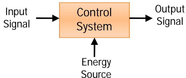
**Open-Loop Control Systems** utilize a controller or control actuator to obtain the desired response.
